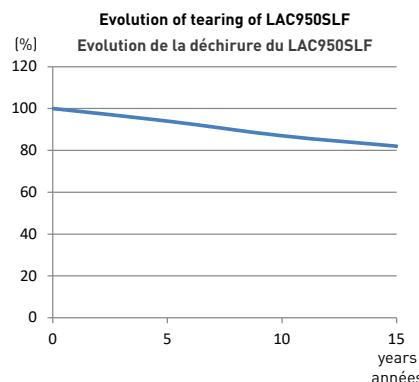
This range of products has undergone accelerated ageing tests (3750h - equivalent to 15 years in the South of France) in the best laboratories and has been shown to maintain its high mechanical performances with very little change in the aesthetic appearance of the material.
