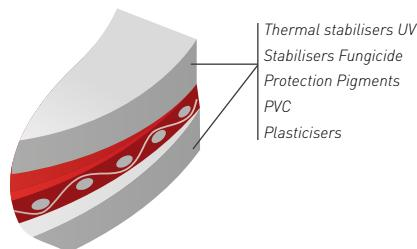
The range of SLF products uses reinforced formulations, optimising resistance to environmental exposure.
