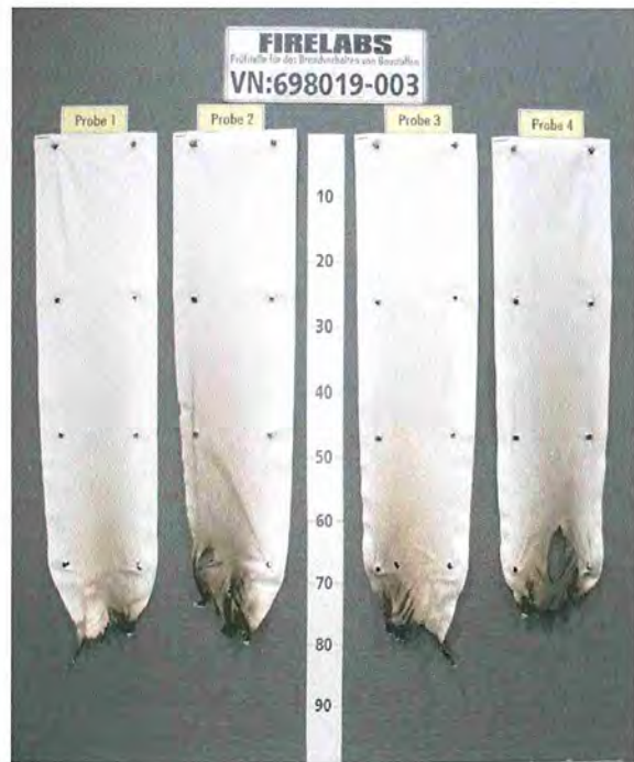
fig. 6 View of test specimen after the test
